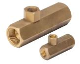
**Pyronics Forced Air Midget Mixers** are suction type proportional air-gas mixers. Air passing through the jet produces a suction in the throat section to entrain a fuel gas. The quantity of gas entrained is easily set by the adjuster plug in the gas throttle cock. Once set, the fuel to air ratio remains constant over a wide range of air flows.
