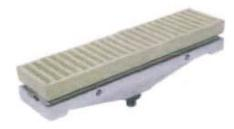
**Pyronics RL-130 Burner** is one of five infrared burners Selas provides for drying/evaporation applications. The Pyronics Infrared Burner is designed primarily for low temperature industrial process heating where heat transfer in the infrared range is highly effective.
