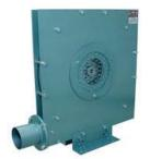
Selas/Pyronics Low Cost (LC) Blowers are used for many industrial and commercial applications requiring air at a specific pressure and volume. The unique design of the single stage unit incorporates a minimum of field maintenance. Sideplates and scroll are steel. Specially designed extruded rubber seals, held tight by tie bolts, prevent leakage. Aluminum impellors, direct connected, provide smooth and quiet operation of the blowers.
