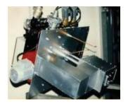
Pyronics Model RSP Series Gas Burner is a pre-packaged, fan-assisted unit designed to suit virtually all types of low temperature gas-fired applications. Typical uses include the firing of industrial ovens and dryers. The RSP can be fitted into process air ducts or installed in process plant recirculation systems. The nozzle mix design, combined with progressive air mixing at the combustion head, ensures that the burner can operate with high turndown capability.
