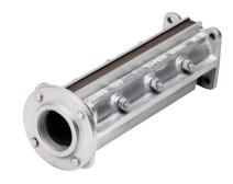
**ERB Water-Cooled Burners** are used for laminating, singeing and drying textiles. These burners were developed for continuous level, direct flame applications where any distortion of the flame pattern would be detrimental to the finished product. This is the only true water-cooled ribbon burner where the cooling core is an integral part of the burner casting and provides maximum flow over the entire burner length.
