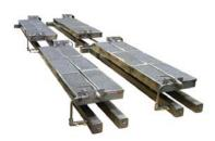
**Red-Ray Apollo Ray Models (AR Series)** are metal fiber surface infrared burners with high radiance and all metal construction. The Apollo-Ray is available in two sizes, 8" x 6" and 12" x 5". Heat capacities are 22,000 btu/hr and 30,000 btu/hr. The radiant output of the burner is approximately 65% IR and 35% convective heat. The emitter temperature reaches 1700° F (927° C) at high fire. The burner is designed to operate most efficiently between 19.1%-19.3% oxygen in the air/gas mixture.
