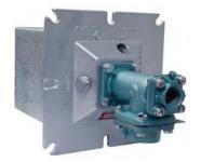
**PYR-HS High Velocity** Hot Shot (HS) series is a nozzle-mixing, high velocity burner used primarily where a high recirculation rate of the products of combustion is required. They produce a high-velocity stream of hot gases at the exit of the burner tunnel which will create a high degree of heat penetration, resulting in greater efficiency and reduced fuel costs. Burners can also operate with excess air or fuel, providing additional versatility in process applications.
