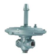
**Balanced Zero Regulator, Model BZR,** is a precise gas flow control regulator for all combustion systems. Used with Proportional Mixers, Nozzle Mix Burners, positive or negative furnace pressures etc. A patented compensator automatically adjusts the valve position to hold constant outlet pressures at all flow rates. The zero regulator will hold the outlet pressure within +/- 2 mm WC over the full range of the turndown.
