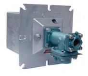
Pyronics XNM Excess Air Burners are nozzle mixing types designed for 800% excess air. Stepped tunnel burner blocks produce excellent flame stability at all firing rates. New air-gas mixing principles produce very high excess air combustion with minimal fumes. All sizes develop maximum ratings with 6 oz. air pressure and 2.5 oz. gas pressure at the burners. All XNM burners feature inconel flame distributors and high temperature refractory blocks. Gas adjustor and flanged connections are standard.
